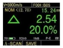
Max/ min mode: This mode shows the current, minimum and maximum thickness values simultaneously for detecting change in material thickness values.
